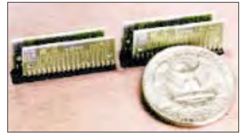
Four substrates on E-Nose each contain eight sensors for detecting toxic compounds.
