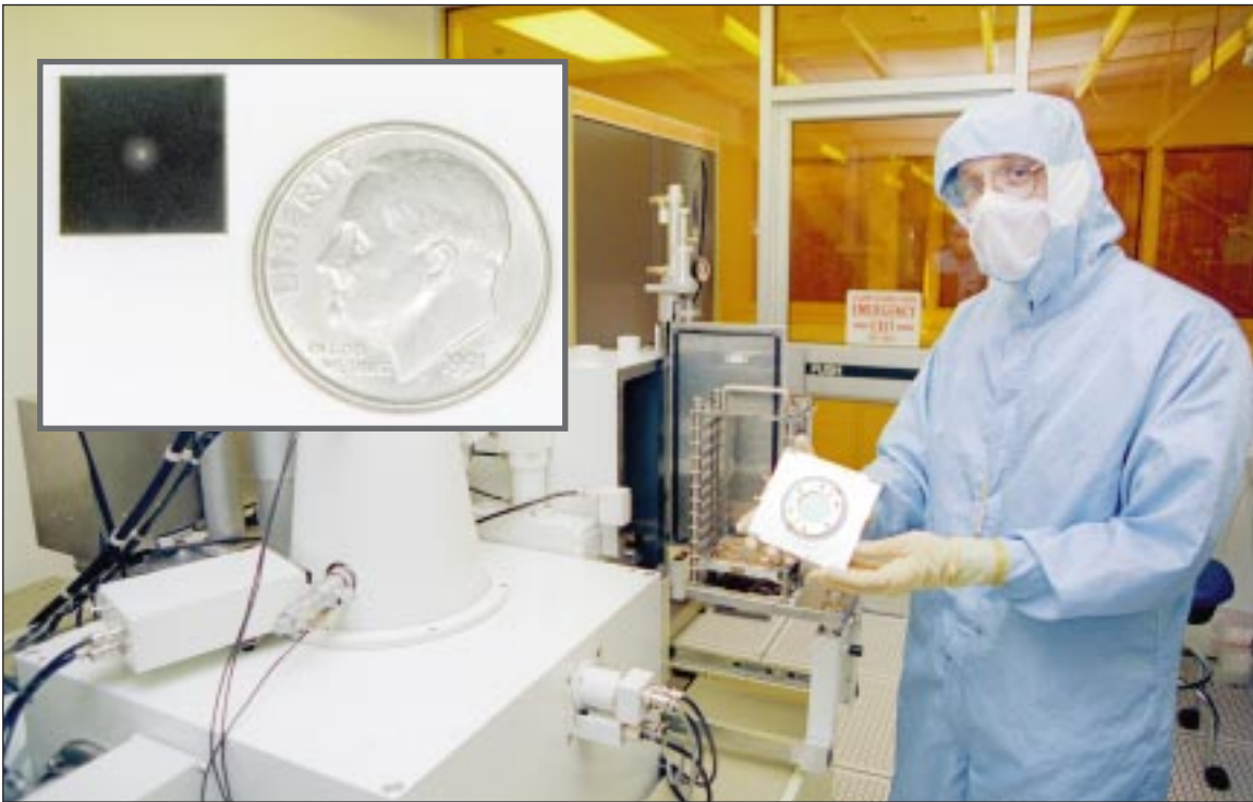
In a Microdevices Laboratory clean room, Dr. Rich Muller of Section 346 prepares electron beam equipment for inscription of names on a wafer that holds a microchip similar to the one shown in inset, which will be engraved with more than 1 million names before it is placed onboard the Stardust spacecraft. For size comparison, the tiny spot in the center of the chip holds about 7,000 names.
