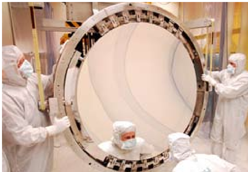
Left: Kepler's primary mirror following the application of reflective coating.
