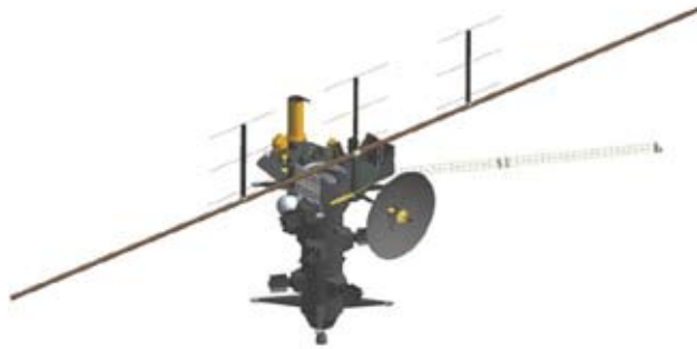
The Jupiter System Observer would study Jupiter and three of its moons before arriving in orbit at Ganymede.
