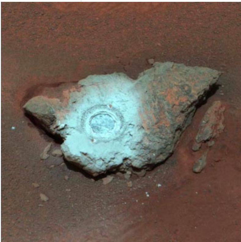
This false-color composite of "Bounce Rock" shows the rock after the Spirit rover drilled into it with its rock abrasion tool. The drilling of the 0.3-inch hole generated a bright powder.
