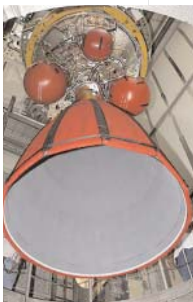
The second stage of SIRTF's Delta II rocket is lowered into position atop the first stage.
