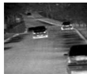
Gunapala, top, shows a wafer holding QWIP sensors used for the newly licensed cancer-screening device and other applications. Above, a QWIP camera image taken at midnight shows where cars were parked earlier in the day as cooler, dark areas.
