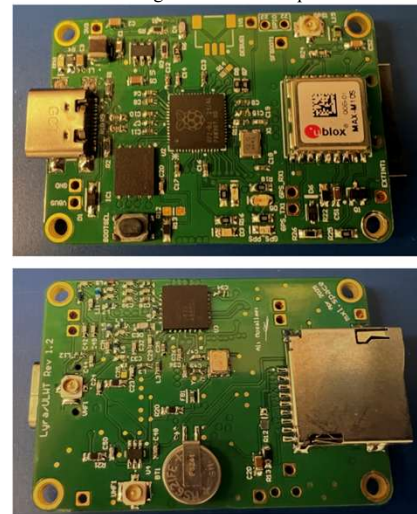
Figure 2 – Embedded hardware for running F-Prime and DTN
