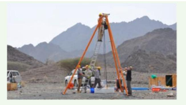
**Figure 1.** Preparing to insert water sampling devices into the subsurface of a serpentinite rock system in Oman, to collect fluids representing extreme chemical and biological conditions.
