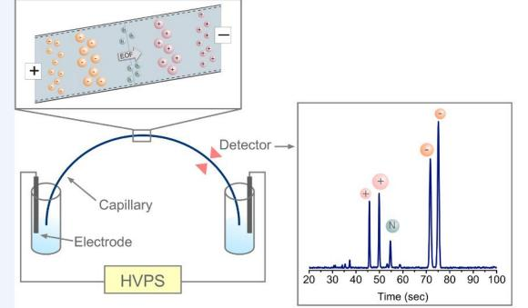
Figure 2. Diagram of a CE system indicating how
