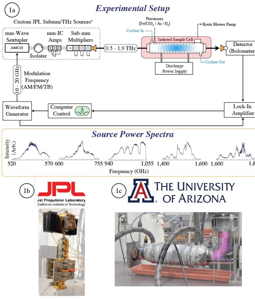
Experimental setup used for frequency modulated direct absorption of transient metal hydrides in block diagram format (1a). The THz radiation sources deployed are supplied by JPL (1b) and interfaced with custom AC/DC glow discharge cells maintained by the Ziurys Group at the University of Arizona (1c).
