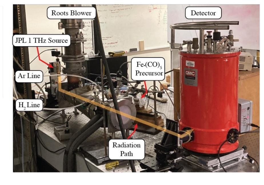
Photograph of the actual experimental setup at the University of Arizona in the Ziurys group research laboratory after the JPL source hardware was transported and installed. Terahertz radiation is columnated with an off-axis parabola and directed through the discharge cell before detection with a liquid helium cooled bolometer detector.
