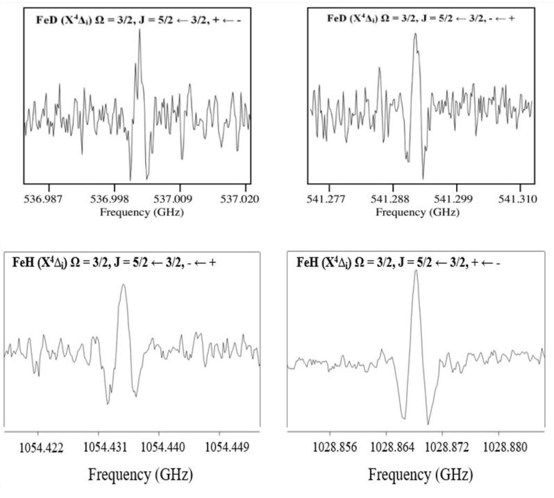
First in class frequency modulated direct absorption measurements of FeH and FeD in the omega = 3/2 and omega = 3/2 ladder.
