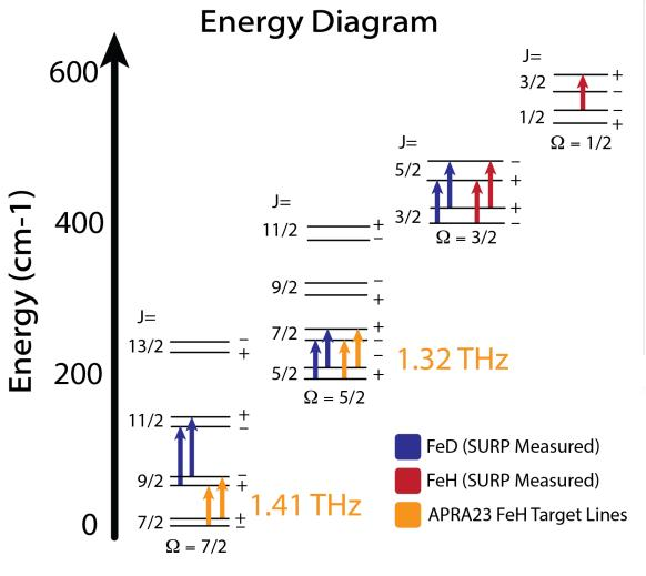
diagram for FeH Energy including all direct absorption lines the University of measured at **SURP** Arizona of part efforts. The experimental highly desirable FeH transitions in the omega=7/2 and 5/2 ladders to be targeted with newly acquired APRA23 funding.
