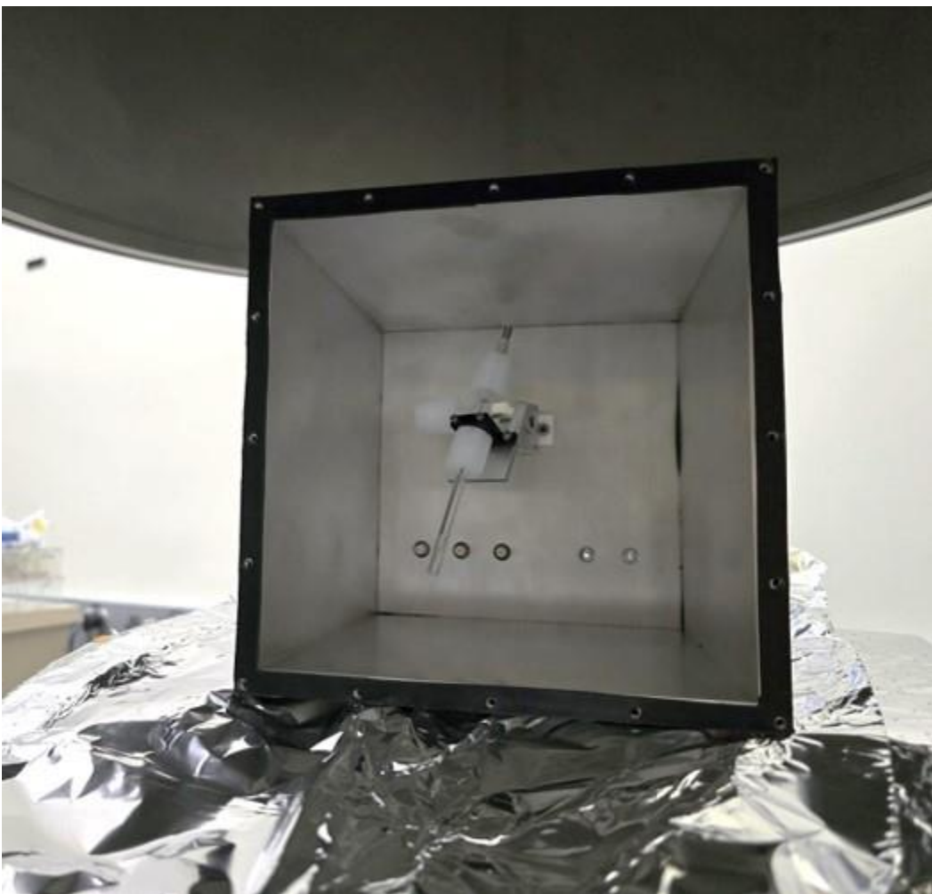
Figure 3. The fabricated and assembled sealed plasma ionization source sitting inside a TVAC.
