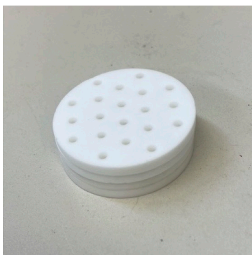
Figure 3 – ceramic discs used to form the cathode array
