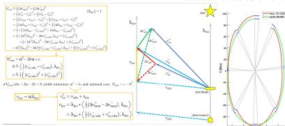
Figure 3: Derivation of Lambert maneuver with relaxation of end velocity along the line of sight. This shows how the projection of the line- of-sight of the Observatory to the star was used to relax just that component of the final arrival velocity. The line-of-sight direction has a wider box than the cross track so the objective was to understand if that could open up the feasibility space and help reduce fuel.
