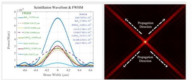
The special resolution parameters, which refer to the FWHM of the beam wavefronts for some scintillators are shown in the left figure. The illustration of the self-collimation in BaF2 PhC is shown in the visual on the right.
