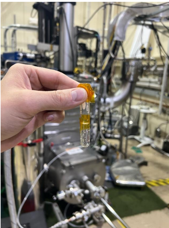
Melted ice in vial measured by Ion Chromatography
