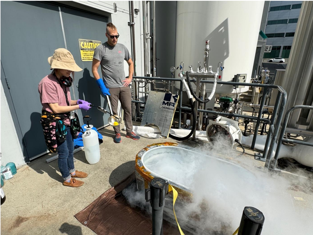
Ice Sample Created by spraying into a bath of liquid nitrogen to create granular ice.
