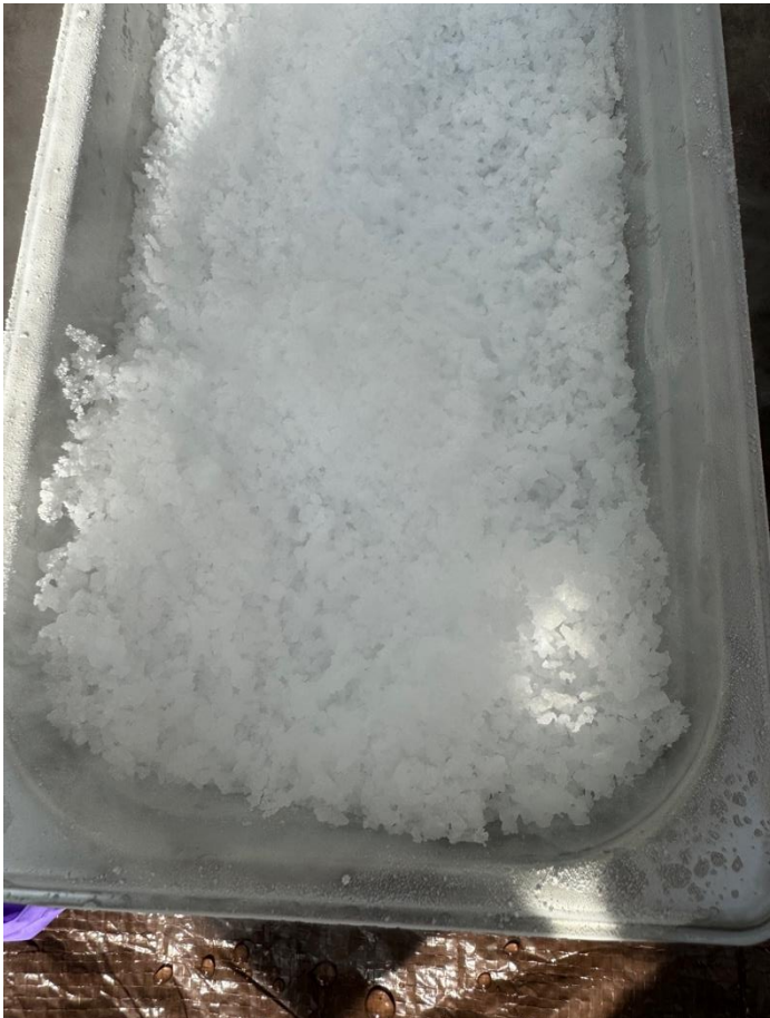
Ice Sample Created by spraying into a bath of liquid nitrogen to create granular ice.
