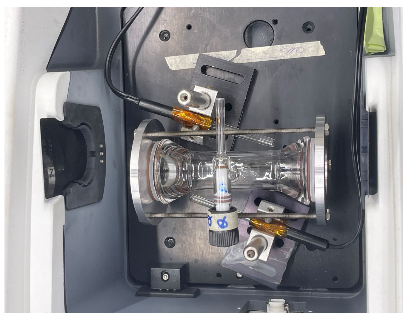
Fig. 2. Photolysis of \text{CO}_2 in a gas cell using two Hg lamps
