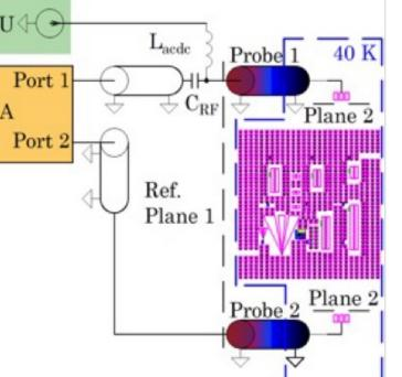
**photograph of the test setup (left) and its diagram (right):** Probe 1 and Probe 2 are room-temperature-to-cryogenic cabling connecting the RF probes and the chip at 40 K to the outside world.
