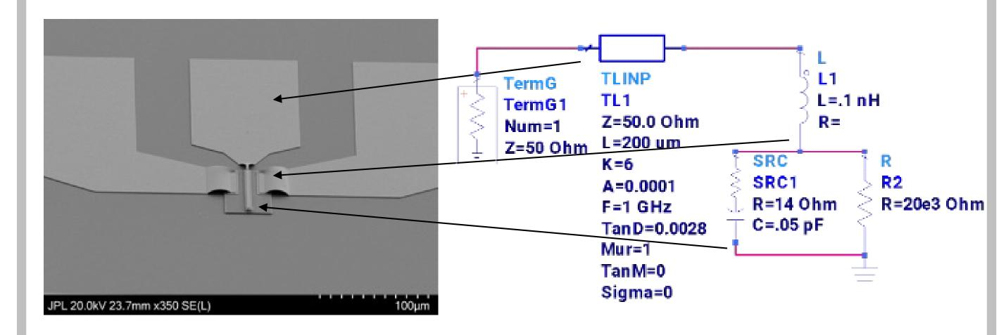
SEM image of the the QWIP and the corresponding electrical circuit model that matches the calibrated amplitude and phase measurements
