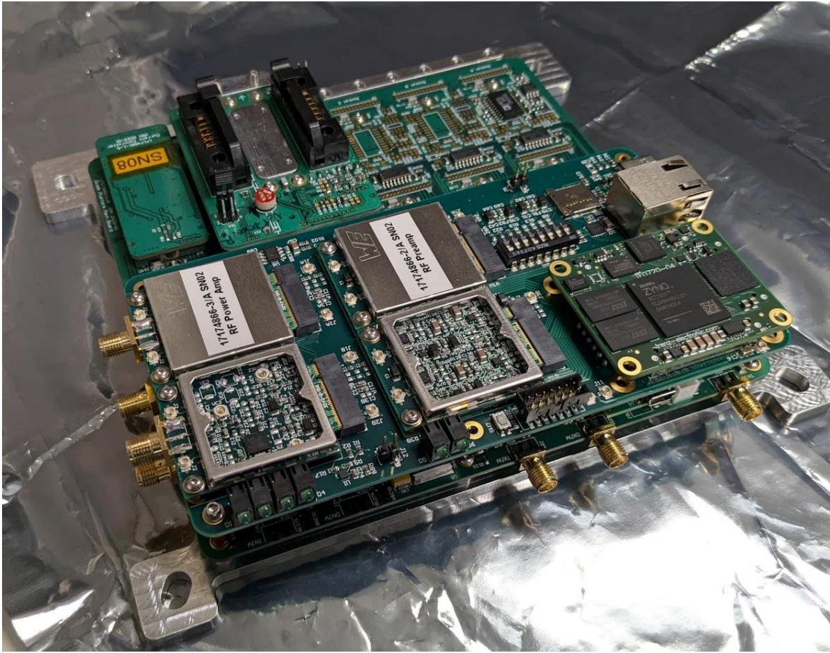
Currently, the new control electronics for the Bragg subsystem are implemented as an add-on mezzanine board, which includes DDS signal generator, preamplifier, and RF power amplifiers to drive two acousto-optic modulators for pulse synthesis.
