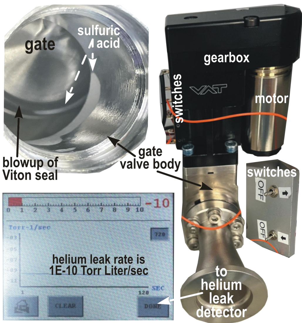
Figure 3. Switch-operated motorized GV (vertical scale 90mm) exposed to 200uℓ of 98% H 2 SO 4 directly on the Viton seal. The measured leak rate was <1E-10 Torr ℓ/s at Patm=760 Torr over 90 days.
