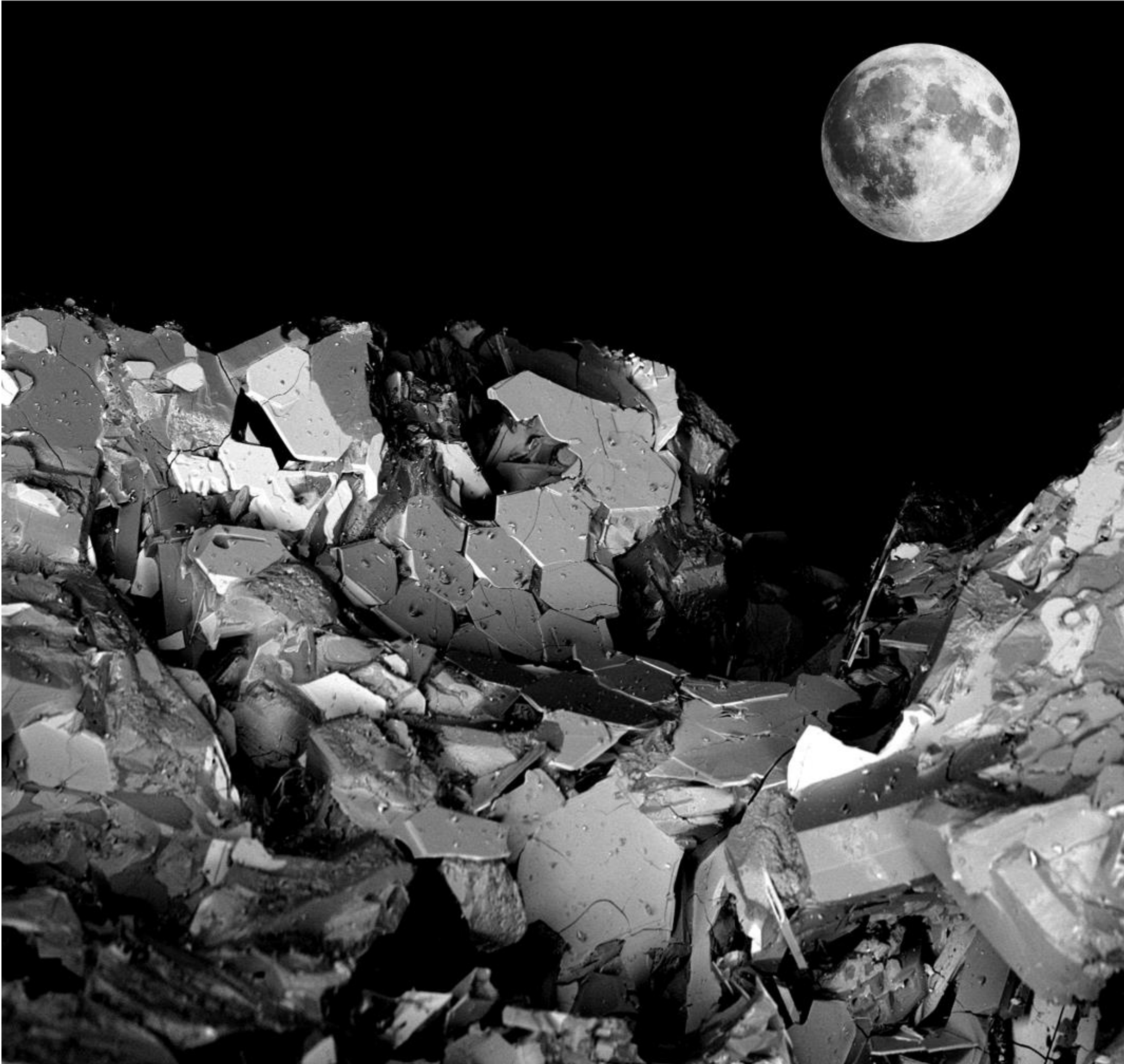
Figure 1: Ilmenite (titanium oxide) crystals in an SEM image of a lunar sample.
