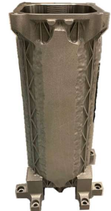
Additively manufactured laser powder bed fusion Ti-6Al-4V topology optimized tank
