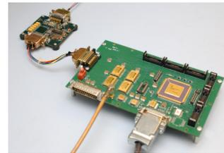
**Figure 4: ISC focal plane (top); MEMS gyro board (middle); DPA electronics (bottom)**
