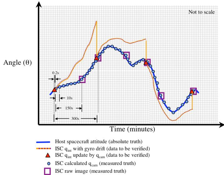
For accuracy validation, two of the three sources of truth are produced by the ISC itself. This concept is referred to as self-score. The ISC attitude quaternion to be validated, shown by the yellow dots in Figure 6, is output at 5 Hz and sent to the ground. In the self-score concept, there are two sources of truth attitude for comparison to the ISC quaternion; ground processed raw images and the ISC camera quaternion.
