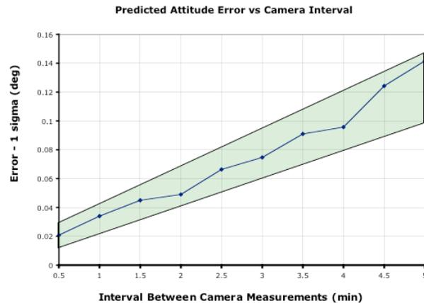
Figure 2: Attitude Error vs. Camera Interval
