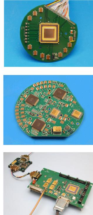
**Figure 4: ISC focal plane (top); MEMS gyro board (middle); DPA electronics (bottom)**
