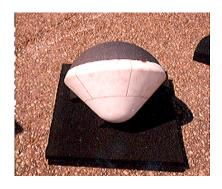
Here is what the NASA engineers decided was the best design for the containers that will protect and keep the Mars Microprobes' right-side-up as they fall through the Martian
