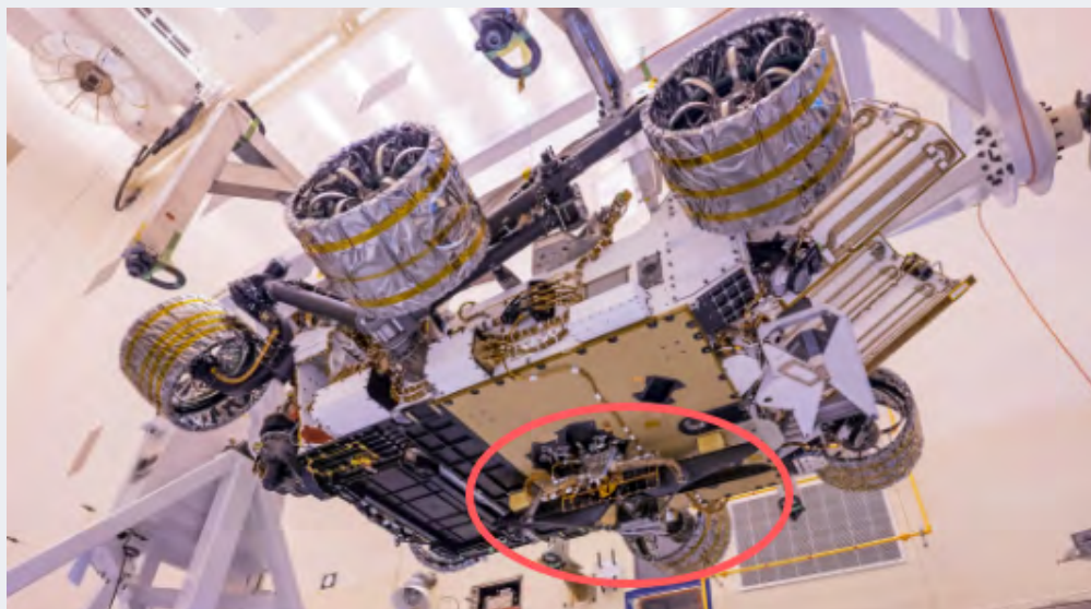
The Mars Helicopter Delivery System holds the Ingenuity Mars Helicopter to the underside of Perseverance | Image credit: NASA/JPL-Caltech
