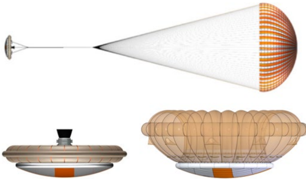
Illustrations of the three new drag devices being developed by the LDSD project: 30-meter Supersonic Disk Sail (SSDS) Parachute (at top), 6-meter SIAD-R (bottom left), 8-meter SIAD-E (bottom right).
