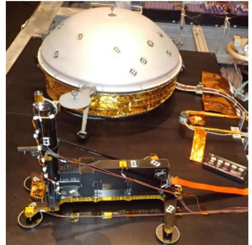
*HP<sup>3</sup> (foreground) and domed Wind and Thermal Shield (covering SEIS) in preparation for thermal vacuum testing. Credit: NASA/JPL-Caltech/Lockheed Martin Space*
