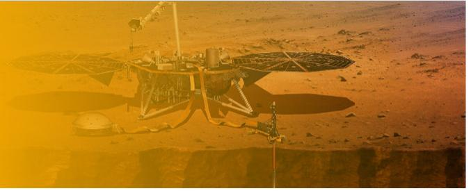
The lander is the core of the InSight spacecraft. Not only will it be the element carrying out all of the activity on Mars, its computer also controls functions of the three secondary elements of the flight system: the cruise stage, back shell and heat shield.
