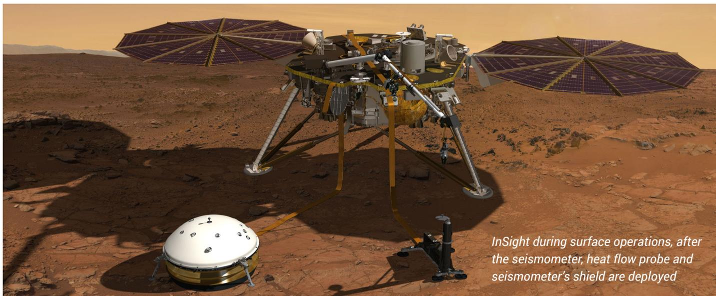
*InSight during surface operations, after the seismometer, heat flow probe and seismometer's shield are deployed*
