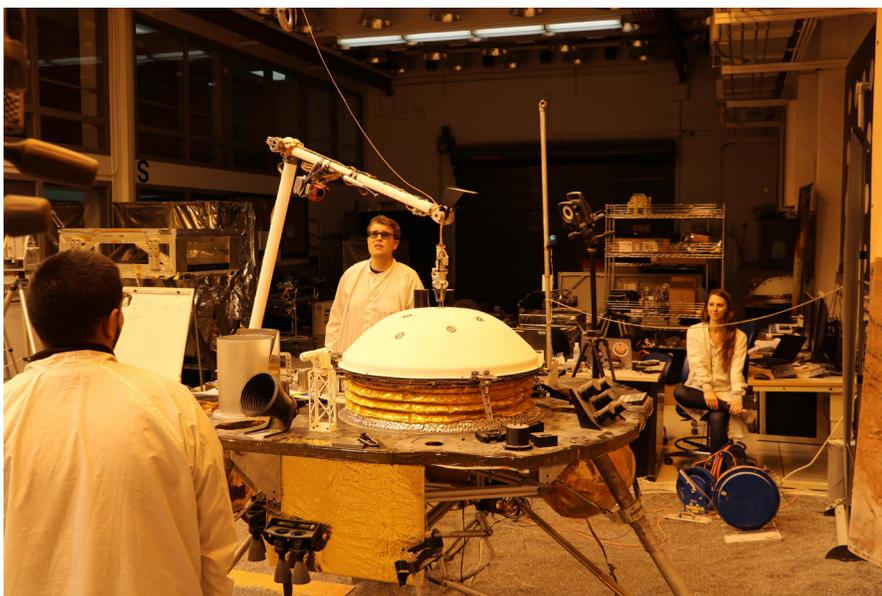
*NASA's InSight mission tests an engineering version of the spacecraft's robotic arm in a Mars-like environment at NASA's Jet Propulsion Laboratory. The Instrument Deployment Camera is visible at the "elbow" of the arm.*
