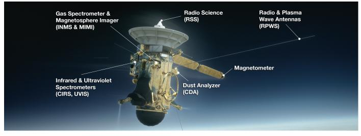
Eight of Cassini's science instruments are planned to be turned on during the final plunge, including the Ion and neutral Mass Spectrometer (INMS). Credit: NASA/JPL-Caltech
