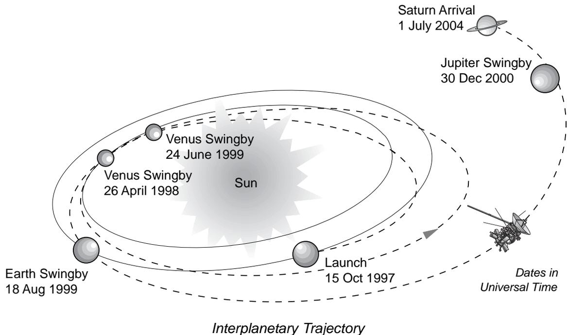
on August 18, 1999. Given these three gravity assists, Cassini finally had enough momentum to reach the outer solar system. The fourth and final gravity assist was from Jupiter on December 30, 2000, at an altitude of 9,723,890 million kilometers (6,042,145 million miles) boosting Cassini all the way to Saturn.
