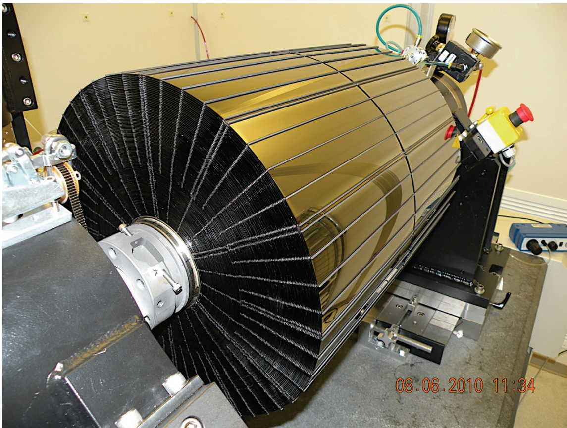
One of two optics units making up NuSTAR's telescope.
