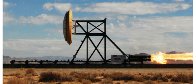
Initial LDSD tests are being conducted using rocket sleds to accelerate the hardware to high speed. This test shows a successful deployment of the SIAD-R decelerator.
