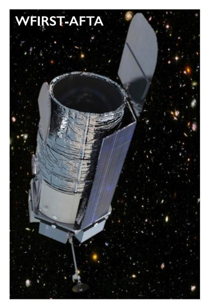
2.4 m TMA ("AFTA") 18 H4RG detectors 0.7 - 2.0 micron bandpass 0.28 sq. deg FoV 4 filter imaging + grism spectroscopy 6 yr. baseline mission
