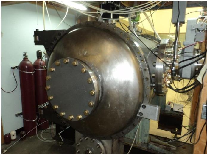
1.2m thermal / ebeam evaporation chamber (Zecoat Corp) with a moving source
