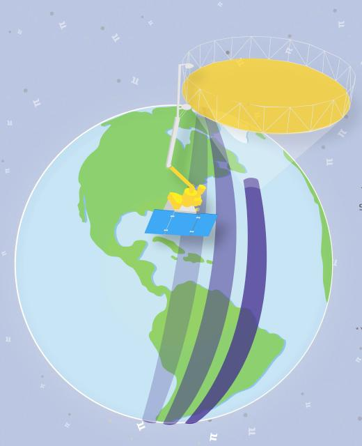
The Soil Moisture Active Passive, or SMAP, satellite is designed to image 1,000-kilometer-wide swaths of Earth from a near-polar, sun-synchronous orbit 685 kilometers above Earth's surface.
