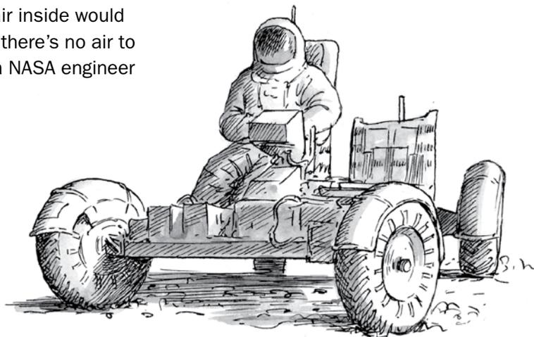
Despite these challenges, engineers designed a tire that worked perfectly when it was used on the moon. It's made of thin bands of springy metal. That helps it be lightweight, have good traction, and work at any temperature the moon can throw
