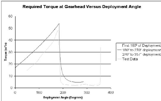
Figure 5. Torque Profile vs. Deployment Angle
