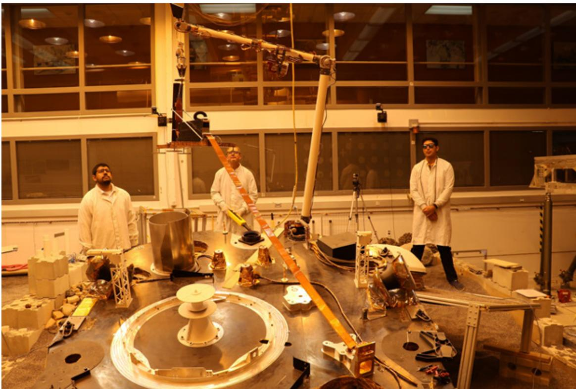
*An engineering version of the robotic arm on NASA's InSight mission lifts the engineering version of the Heat Flow and Physical Properties Probe (HP<sup>3</sup>) at NASA's Jet Propulsion Laboratory.*
