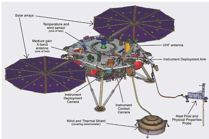
The lander's panels are based on the design of those flown on NASA's Mars Phoenix Lander, though InSight's were made slightly larger for more power output and to increase structural strength. These changes were required to support the two-year landed prime science mission with sufficient margins (two Earth years, one Mars year).
