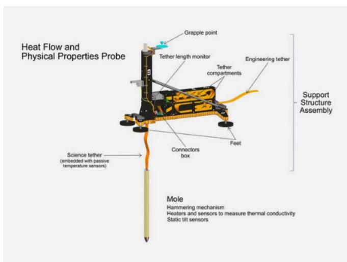
*Illustration of InSight's HP<sup>3</sup> instrument with some key components labeled.*
