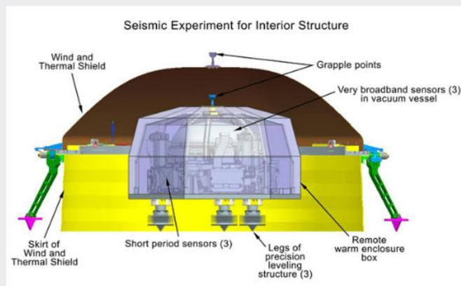
*Illustration of InSight’s SEIS instrument with some key components labeled*
