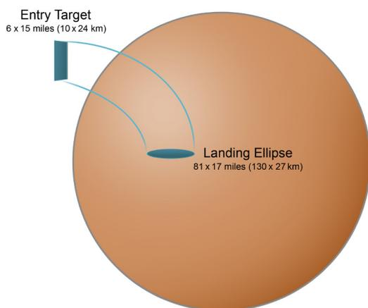
*Navigators' target at the top of Mars' atmosphere is smaller than the ellipse covering the area in which the spacecraft has a 99 percent chance of touching down after passing through that target. Dispersion factors include aerodynamic uncertainties and atmospheric variability. This concept illustration is not to scale.*
