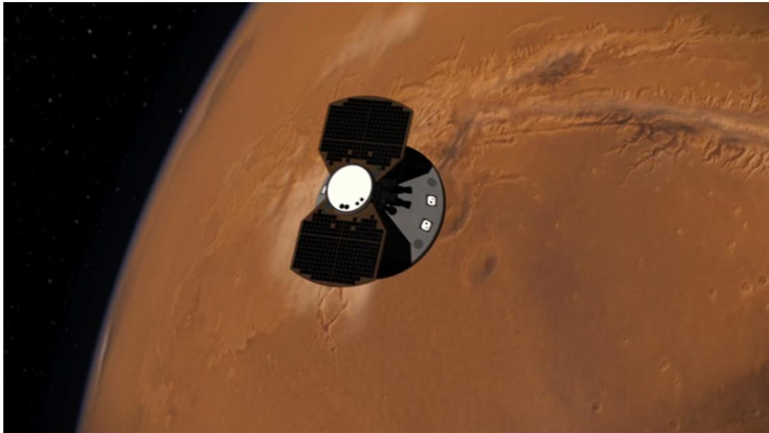
After launching on May 5, 2018, InSight began a 6.5-month cruise through space. On Nov. 26, it will hit a target point at the top of the Martian atmosphere at about six times the speed of a high-velocity bullet. It will then begin a process known as entry, descent and landing: It will decelerate enough in 6.5 minutes for a safe touchdown on Mars, deploying its three legs to absorb its impact on the Martian surface.
