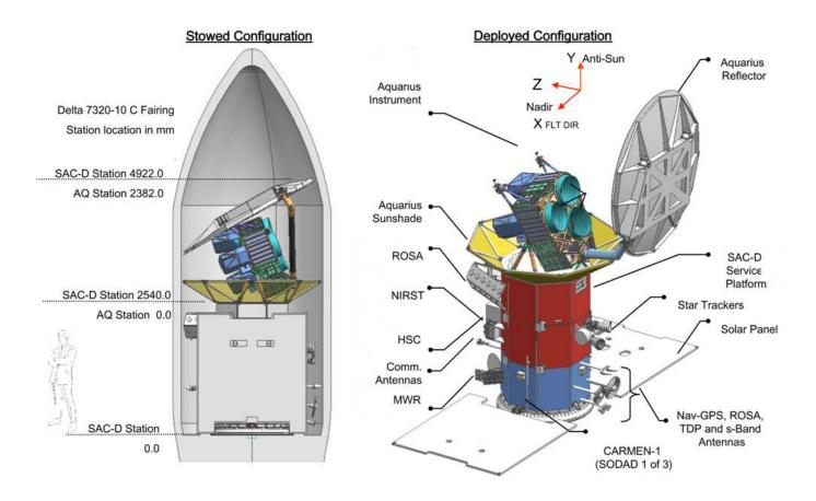
Aquarius will achieve its highly accurate ocean surface salinity measurements through three primary methods: averaging co-located data sets, performing on-orbit calibrations, and maintaining thermal stability of the key instrument subsystems. Data averaging every seven days and every month will be a ground processing activity.
