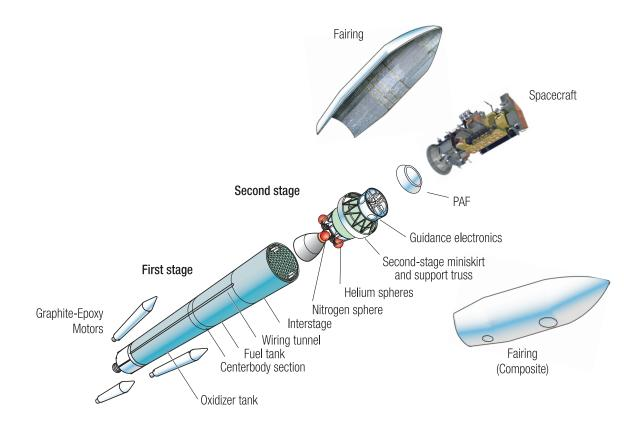
The first stage of the Delta II uses a Pratt & Whitney Rocketdyne RS-27A main engine. The engine provides nearly 237,000 pounds (1,054,229 newtons) of thrust by reacting RP-1 fuel (thermally stable kerosene) with liquid oxygen.
