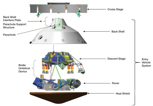
Mars Science Laboratory flight system, expanded view
